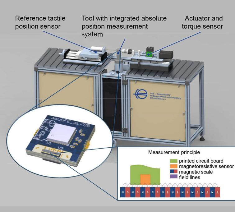
Measurement System using absolute position sensor for referencing of small, relative position sensors which are integratable for small space, low-cost applications.
